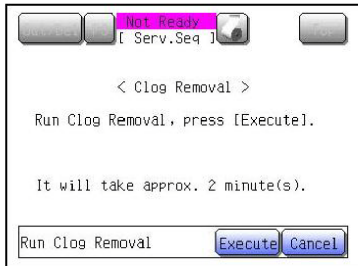
"Run Clog Removal" Screen
